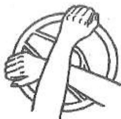
One hand pushes the steering wheel up, across and down, while the other hand reaches up to the top of the wheel and pulls down. This action is repeated, grasping the wheel at the top again.
